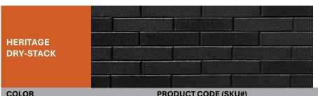
Heritage Dry-Stack is a mortarless clay brick veneer that features a rolled edge. Each brick is approximately 11.625" in length, 2.75" in height and 1.6" thick. Coverage is based on tight-fit joints and 4.5 bricks make up 1 sq. ft. Coverage will vary based on joint size, cutting or trimming preferences. 1 clip required per brick.
