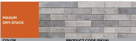
Maxum Dry-Stack is a concrete brick veneer that features a bevelled edge. Each brick is approximately 15.3" in length, 3.5" in height and 1.8" thick. Coverage is based on tight-fit joints and 2.6 bricks make up 1 sq. ft. Coverage will vary based on joint size, cutting or trimming preferences. Use one clip per brick for walls under 30 feet high and two clips per brick for walls 30 feet and taller.
