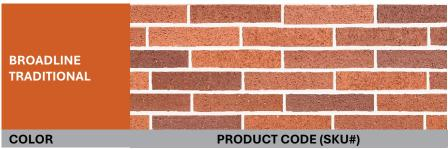
Broadline Traditional is a mortared clay brick veneer that features a square edge. Each brick is approximately 11.625" in length, 2.75" in height and 1.6" thick. Coverage is based on ½" joints and 3.9 bricks make up 1 sq. ft. Coverage will vary based on joint size, cutting or trimming preferences. 1 clip required per brick.
